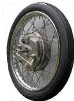
Norton Wheel with Custom Triumph TLS Brake
